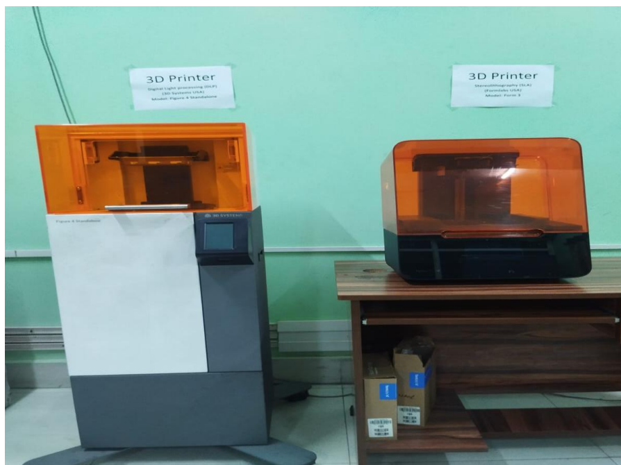
3D PRINTER Digital Light Processing (DLP) (3D Systems USA) Model Figure 4 Standalone
